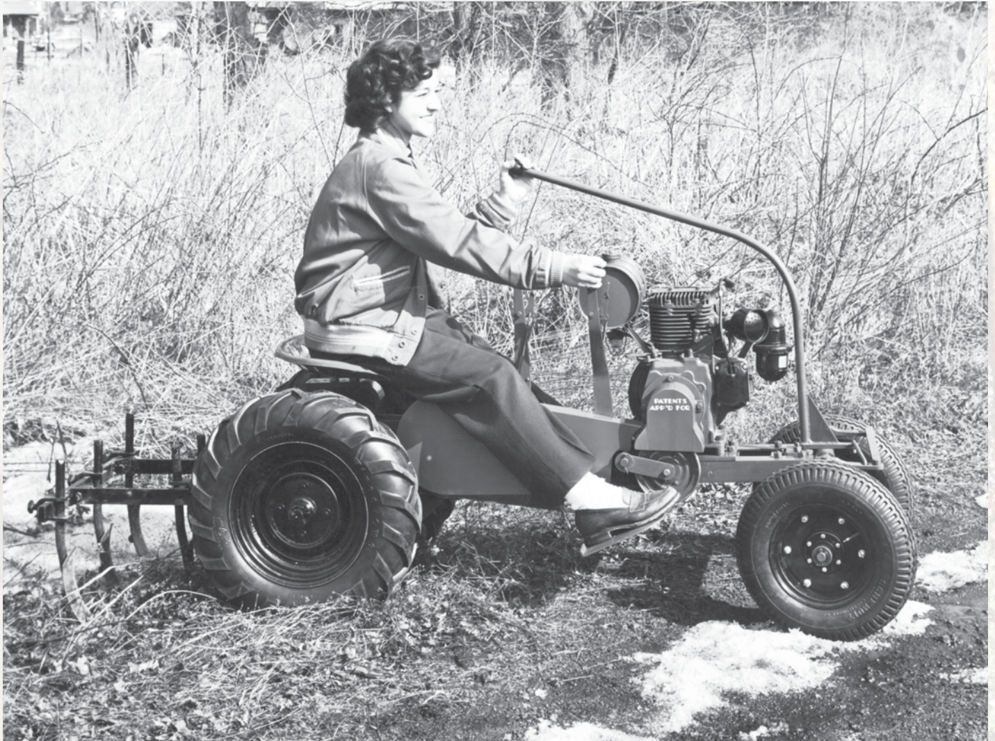
This is the earliest known picture of the prototype built by Arthur J. Lewis II. This picture was taken behind the Baird factory. Notice that the engine belt guard is a weldment. The lady operating the tractor is believed to be Rita Wilkerson from Baird's accounting department. She started with the company in 1937.
